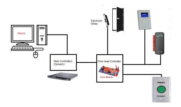
Figure 14 – Typical Security Control Schematic
