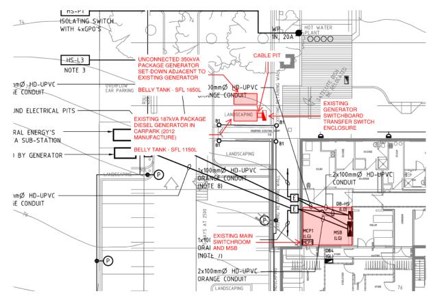
Figure 6 Existing Generator System Locality Plan
